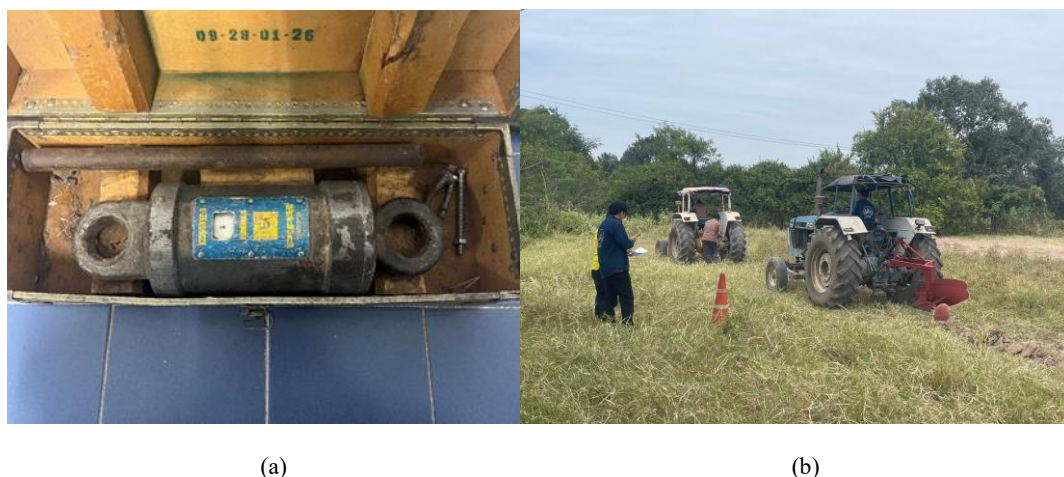
Figure 2 Traction force measurement: (a) Dynamometer (b) During traction force measurement
