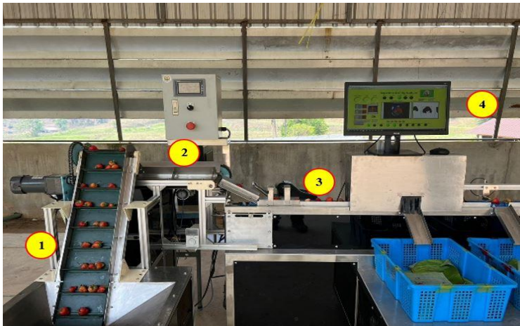
Figure 9 Prototype components of strawberry sorting machine using image processing technique
