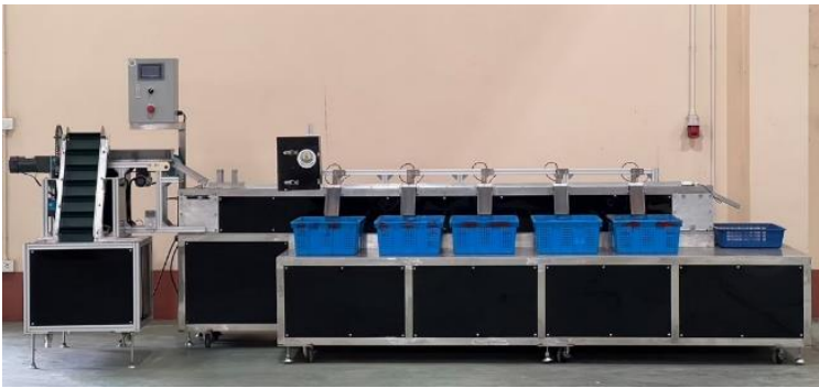
Figure 8 Prototype of strawberry sorting machine using image processing technique
