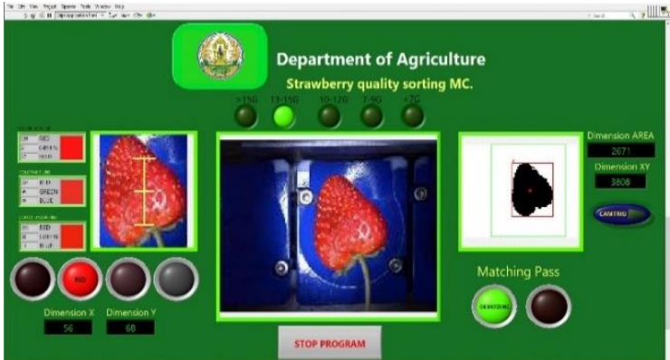
Figure 9 Prototype components of strawberry sorting machine using image processing technique
