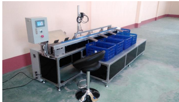
Figure 3 Preliminary prototype of strawberry color sorter using Image Processing technique
