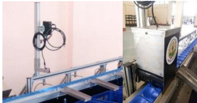
Figure 4 Install the camera cage on the sorting belt before adjustment (Left) after adjustment (right).
