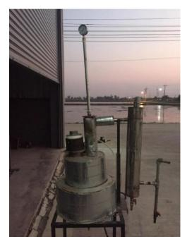
Figure 1 A pyrolysis furnace for the test
