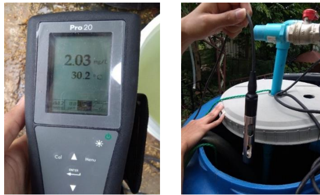
Figure 3 OD measurement of water in a holding tank
