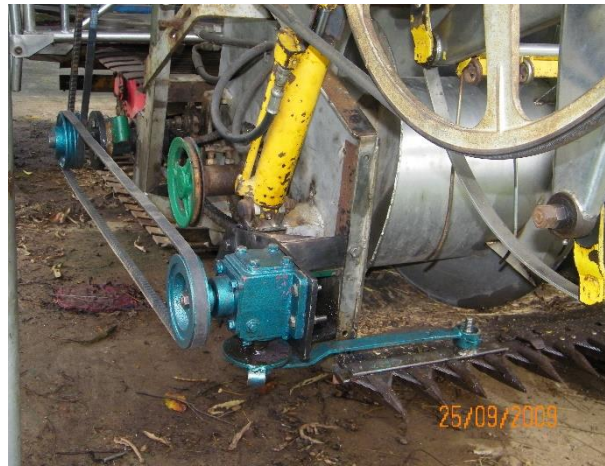
Figure 4 Perpendicular axis type driven by the belt
