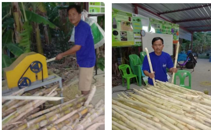
Figure 5 The actual operation of a sugarcane abrasive machine by a farmer.
