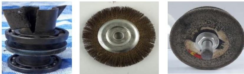
Figure 1 The blade types; a) Knife blade, b) Wrie brush and c) Abrasive stone.
