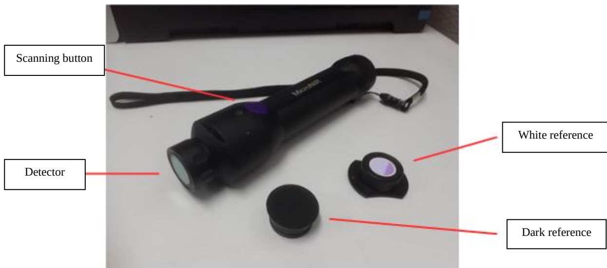
Figure 1 Micro-NIR spectroscopy, Onsite – W model, VIAVI solutions, USA.
