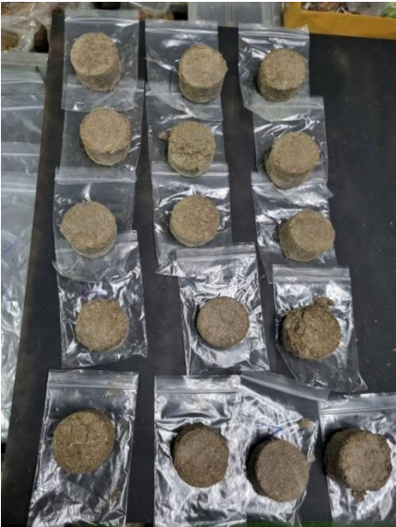
Figure 1 Sugarcane leaf pellet samples with varying levels of impurities (sand)
