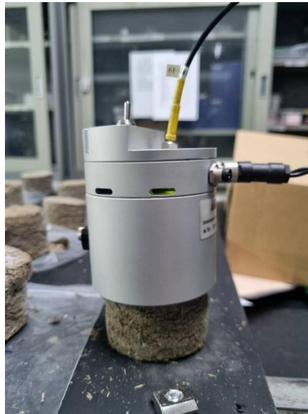
Figure 2 Spectral measurement setup using a fiber optic probe coupled with an integrating sphere
