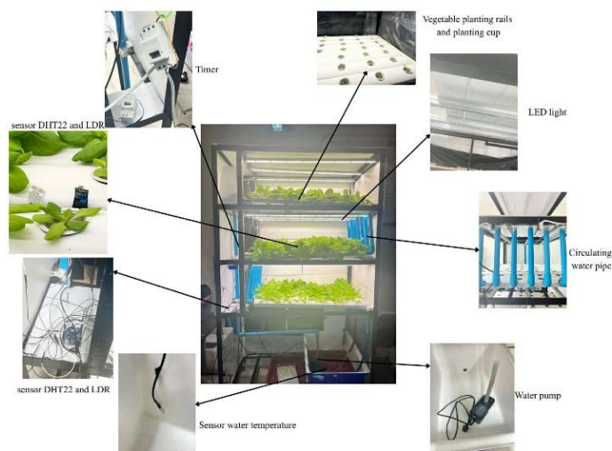
Figure 3 Structure of the framework used for cultivating butterhead, including sensors, lighting, water circulation
