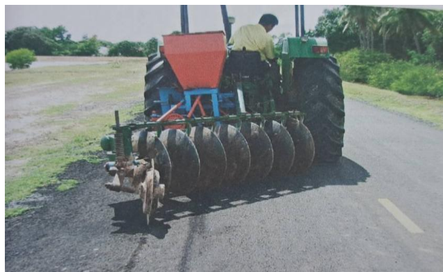
Figure 1 The rice seeder combined with a 7-disk plow on a concrete
