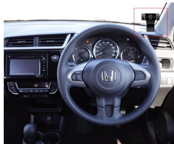
Fig. 2 Camera placement for driver drowsiness detection
