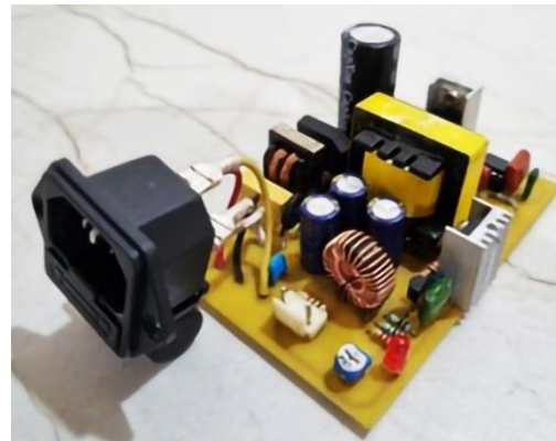
Figure 5. Compact 24 V, 2.5 A, 60 W final working prototype of the SMPS
