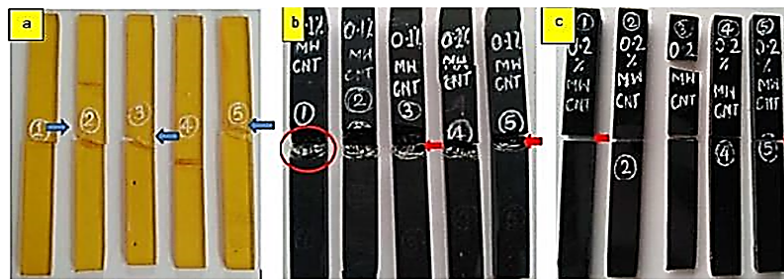
Figure 10. Specimens after flexural testing: (a) Neat epoxy; (b) 0.1% MWCNTs; (c) 0.2% MWCNTs
