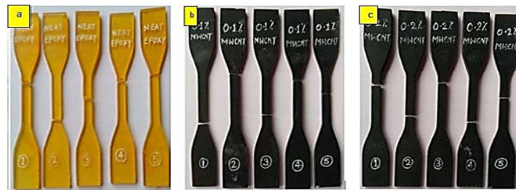
Figure 8. Specimens after tensile testing: (a) Neat epoxy; (b) 0.1% MWCNTs; (c) 0.2% MWCNTs
