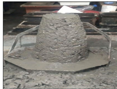
Figure 6. Slump Test for fresh concrete
