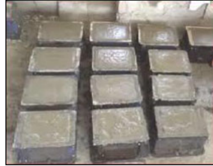
Figure 5. Permeable paver block Specimens
