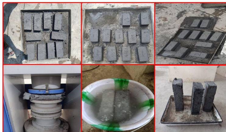
Figure 4. Casting and Testing of Papercrete Specimen
