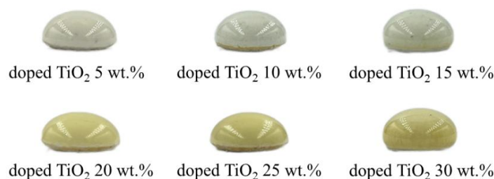
Figure 1. Side view images of the glass ceramic composites with concentrations of \text{Ti}_{0.98}(\text{Ni}_{0.01}, \text{Nb}_{0.01})\text{O}_2 ceramic ranging from 5-30 wt%
