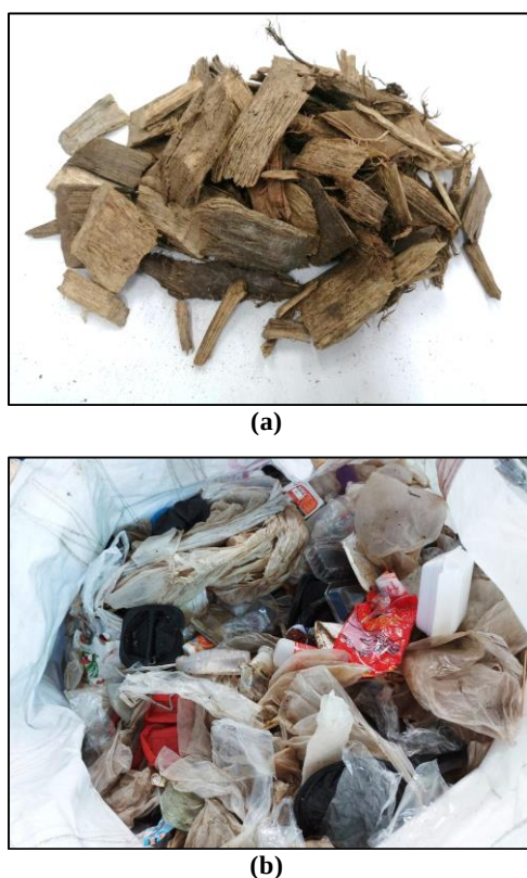
Figure 1. Images of (a) Woodchips (b) RDF-3
