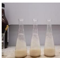
Figure 2. Hydrolysis preparation of cassava peel using H 2 SO 4
