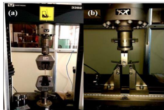
Figure 4. Loading arrangement for (a) Tensile test; (b) flexural test
