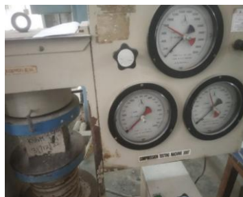
Figure 3. Shows compressive strength test on 300 T CTM
