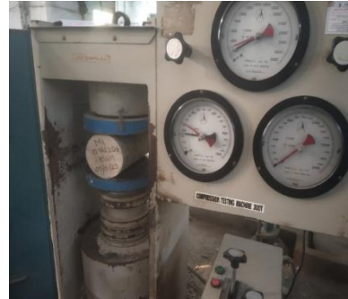
Figure 5. shows split tensile strength test using 300 T CTM
