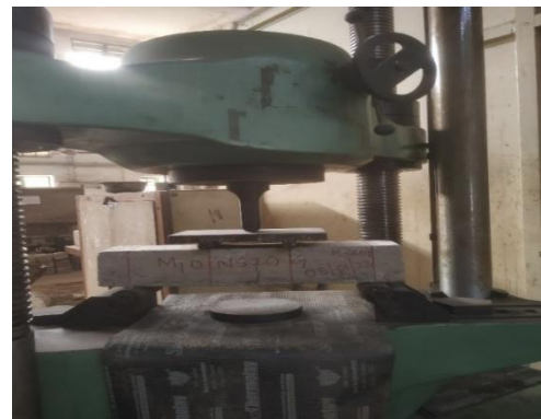
Figure 7. shows flexural strength test using 100 T UTM
