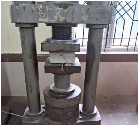
Figure 6. Split Tensile test Image
