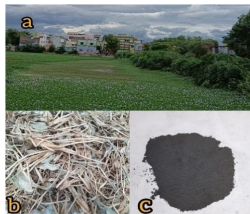
Figure 1. a) Water Hyacinth Residues, b) Dried Biomass, and c) Biomass Ash
