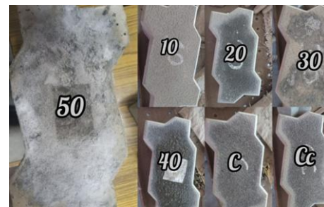
Figure 14. Efflorescence the paver block (WHA 50%)
