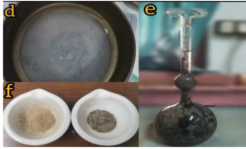
Figure 2. d) Fineness, e) Ignition, and f) Specific Gravity
