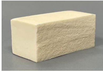
Figure 1. The appearance of the dissected fully cured NRLF prepared using microwave irradiation power and time of 600 W and 6 mins, respectively
