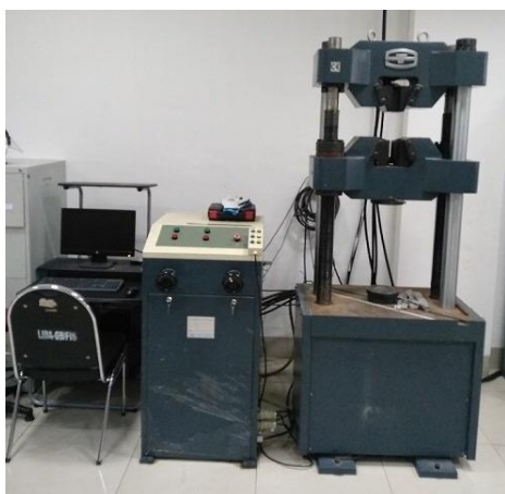
Figure 2. Compressive strength test equipment type UTM WEW-300D
