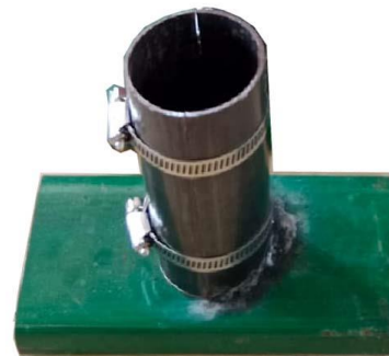
Figure 1. CCC specimen mold based on ASTM C39 standard
