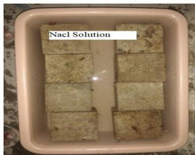
Figure 6. Specimens submerged in 5% HCL solution
