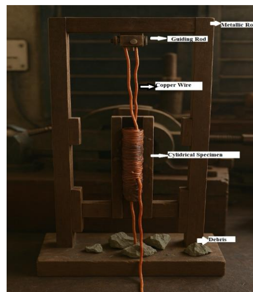
Figure 10. Impact Test on Cylindrical Disk
