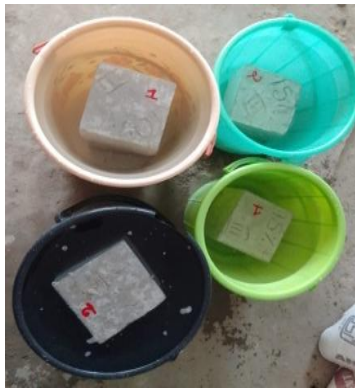
Figure 8. Water absorption test on cubes
