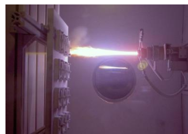
Figure 3. Plasma spray coating of ceramic coating onto a metal substrate
