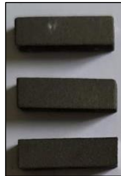
Figure 2. Scratch test specimen of 8, 10, 12% SiC for 100 µ coating thickness
