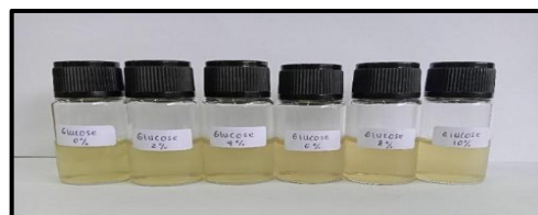
Figure 7. AgNP nanocolloidal solutions containing glucose with different concentrations
