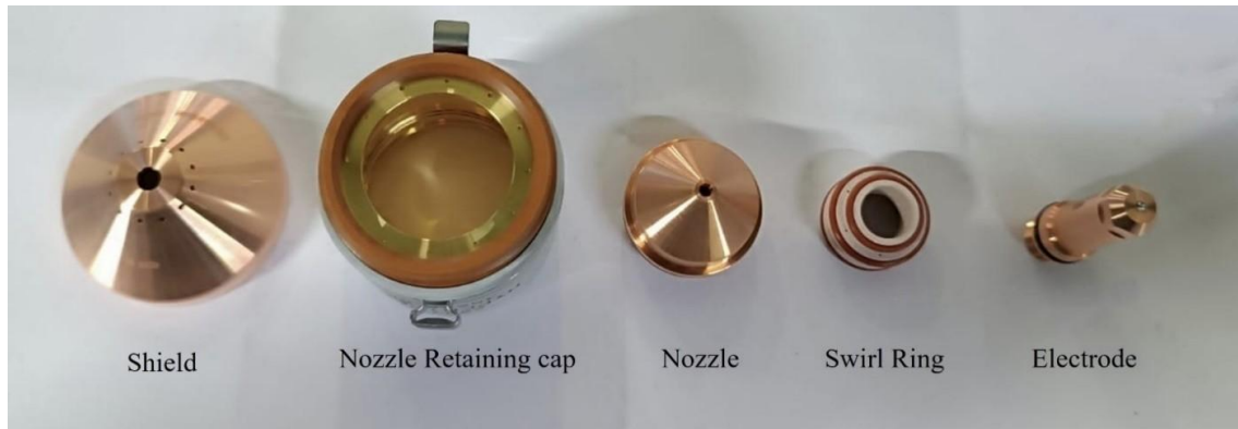
Figure 2. Air consumable 200 A plasma cutting nozzle and torch parts
