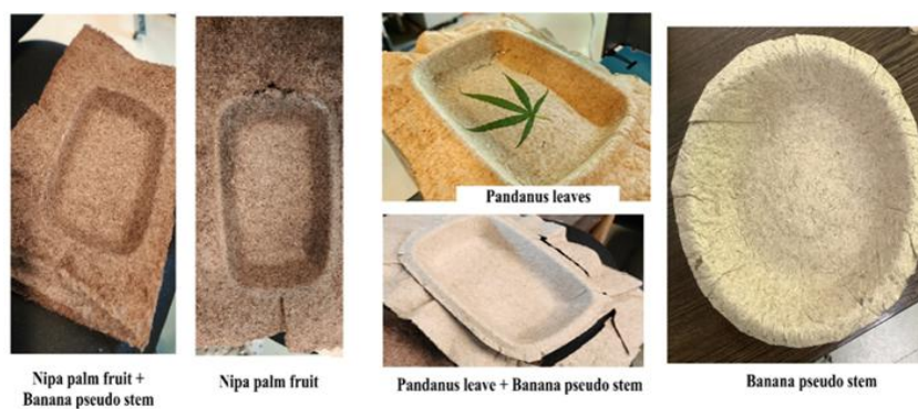
Figure 4. Paper containers made from Nipa palm fruit, pandanus leaves, banana pseudo stem, and the mixed paper sheet
