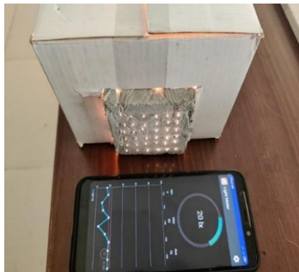
Figure 4. Light transmittance and measurement of lux values
