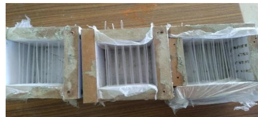
Figure 2. Weaving of optical fibres
