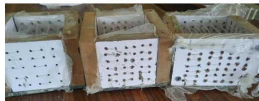
Figure 1. Arrangement of plastic fibre optic cable for (5×5), (6×6), (7×7) densities
