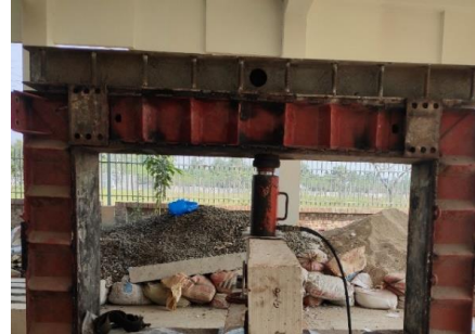
Figure 6. Shows experimental setup for beam load test
