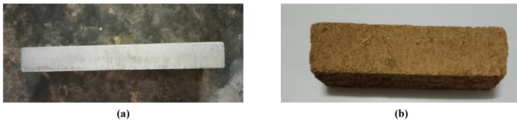
Figure 8. Physical characteristics and thermal properties of (a) Lightweight concrete \Delta x=75 \text{ cm} , k=0.18 \text{ w/m}^\circ\text{C} , \rho=620 \text{ kg/m}^3 , C_p=0.84 \text{ kJ/kg}^\circ\text{C} , and (b) Hemp concrete \Delta x=75 \text{ cm} , k=0.14 \text{ w/m}^\circ\text{C} , \rho=1,008 \text{ kg/m}^3 , C_p=1.02 \text{ kJ/kg}^\circ\text{C}
