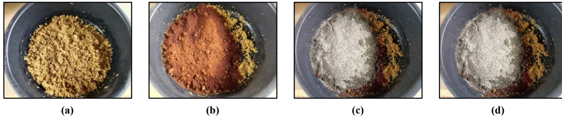
Figure 3. Process for Hemp Concrete Production: (a) Hemp soaked in water with dissolved \text{Al}_2(\text{SO}_4)_3 for 5 minutes (b) Soil added and mixed thoroughly (c) Hydraulic cement added and (d) Water mixed with polymer added and mixed thoroughly
