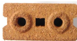
(d) Hemp Concrete (HC-15A); \Delta x = 125 \text{ cm} , k = 0.16 \text{ w/m}^\circ\text{C} , \rho = 1,260 \text{ kg/m}^3 , c = 1.24 \text{ kJ/kg.C}
