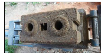
Figure 6. Example of hemp concrete formed using an interlocking block-making machine
