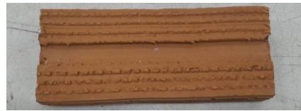
(a) Red Brick; \Delta x = 65 \text{ cm} , k = 0.47 \text{ w/m}^\circ\text{C} , \rho = 1,600 \text{ kg/m}^3 , c = 0.79 \text{ kJ/kg.C}
