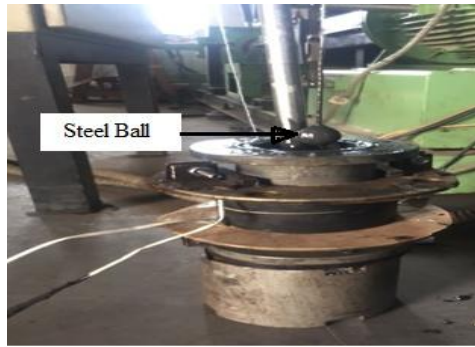
Figure 11. Viscosity measurement setup
