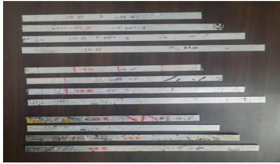
Figure 1. The fabricated 2/1 configurations FML (AL/GF-E/AL) composite beams
