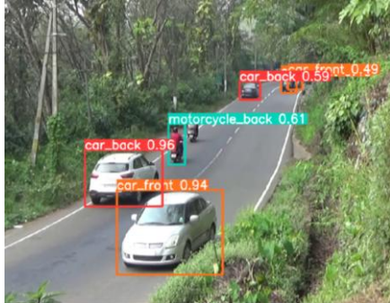
Figure 8. Shows Detection of Vehicles Using Vehicle Orientation Dataset
