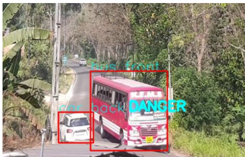
Figure 11. Shows Detecting the Dangerous Vehicle Coming into The Curve
