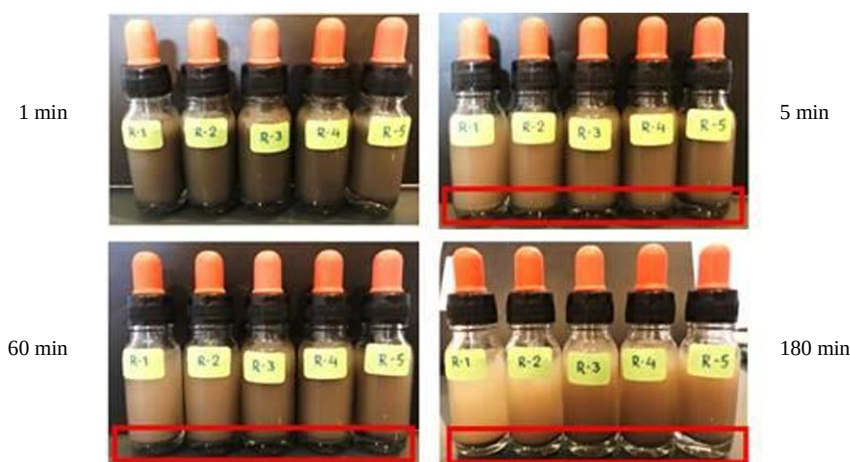
Figure 2. Precipitation of rice husk ash (4% by weight) suspended in water 1, 5, 60, and 180 min
