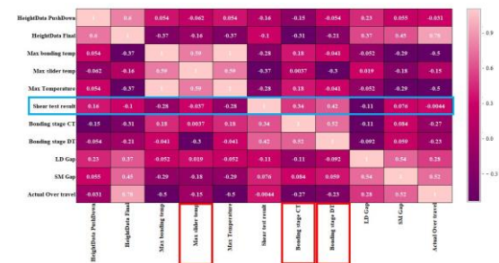
Figure 4. Heat map correlation technique for shear strength of Au-Sn (IMCs) joint
