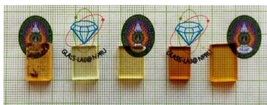
Figure 1. The picture of a series of glass samples with varying concentrations of \text{Dy}_2\text{O}_3 , arranged from left to right in order of increasing concentration (0.0, 0.1, 0.5, 1.0, and 1.5 mol%)
