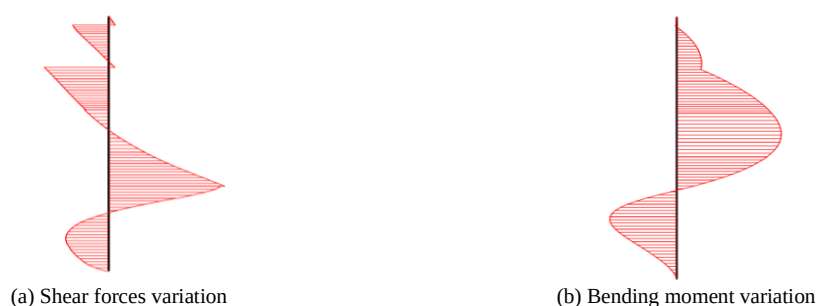
Figure 10. Variation of shear and bending forces in diaphragm wall with multiple i-section strut member
