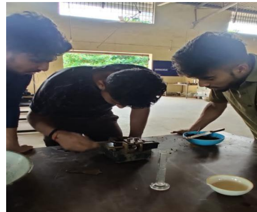
Figure 10. Performing Liquid Limit Test
