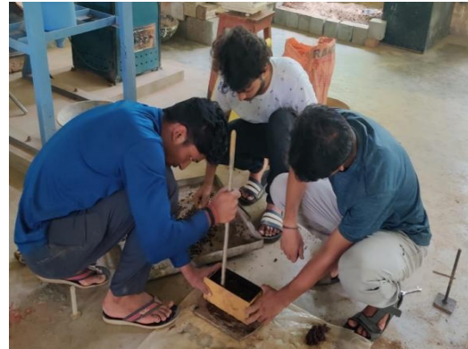
Figure 9. Casting of SMB
