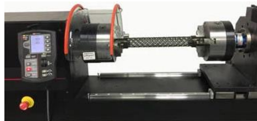
Figure 3. Torsion Testing of Composite Drive Shaft (Lenwari et al. , 2022)
