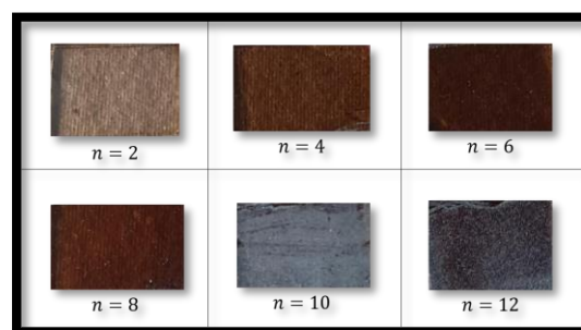
Figure 1. Spin-coated cobalt ferrite of two(n=2)to twelve (n=12) layers Structural Studies
