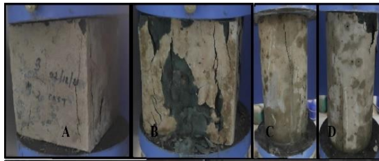
Figure 8. Failure pattern of specimens
