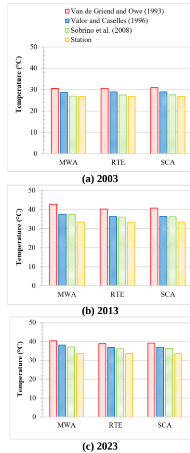
Figure 2. Comparison of LST determined using satellite data of the years - (a) 2003, (b) 2013 and (c) 2023 respectively with weather station data by using different LSE models
