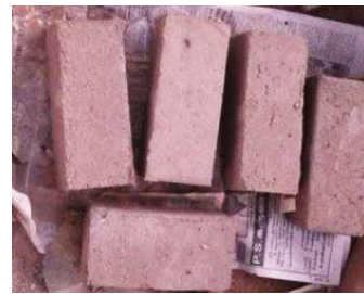
Figure 2. Fly ash based geopolymers bricks (Subramani et al. , 2016)
