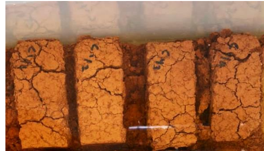
Figure 9. LAT 1-based controlled brick sample after 24-hour water absorption test
