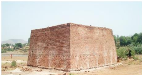
Figure 1. A typical clamp-form brick kiln in Karad, India (Kulkarni and Rao, 2016)
