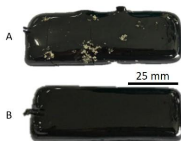
Figure 3. Images of the cast (A) BP glass and (B) BL glass, both melted at 1300^\circ\text{C} . (A) The glass shows large regions of grey discolorations. (B) The glass is free of discolorations
