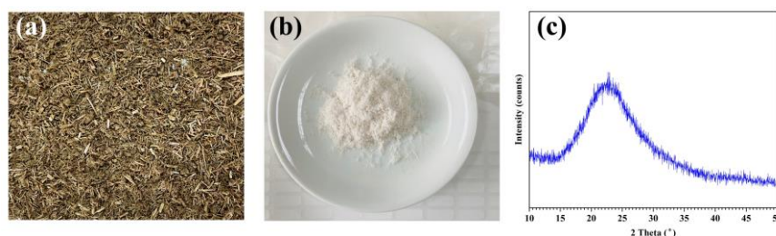
Figure 1. Texture appearance of sugarcane leaves: (a) after leaching with 2.0 M HCl; (b) after calcination and (c) XRD pattern of solid powder after acid leaching and calcination
