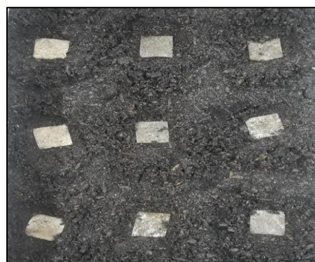
Figure 4. Images of samples for biodegradability test
